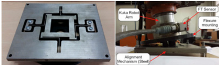
Fig. 4: A compliant 5-DOF flexure based passive gripper integrated with Kuka robot for pick-and place and insertion task [5].
