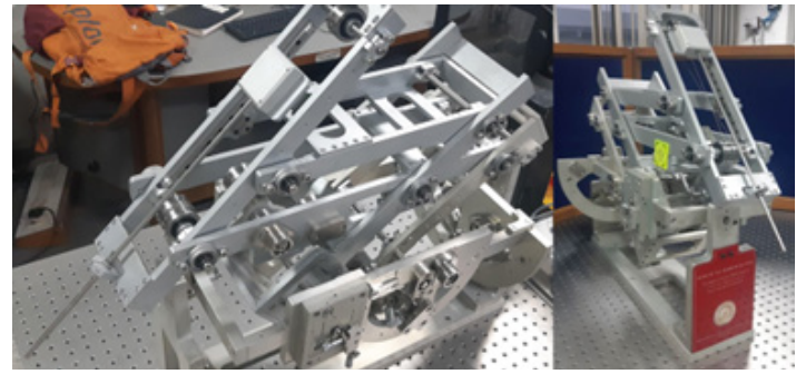
Fig. 5: Remote Centre of Compliance Manipulator for robot-assisted minimally invasive surgery. A compliant mechanism is used to facilitate adjustment post assembly [6].
