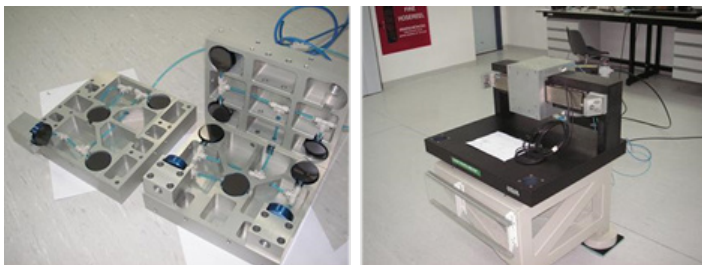
Fig. 1: Assembly of porous air bearings. Linear motors and air bearings used in developing ultra-precision motion stage [1].
