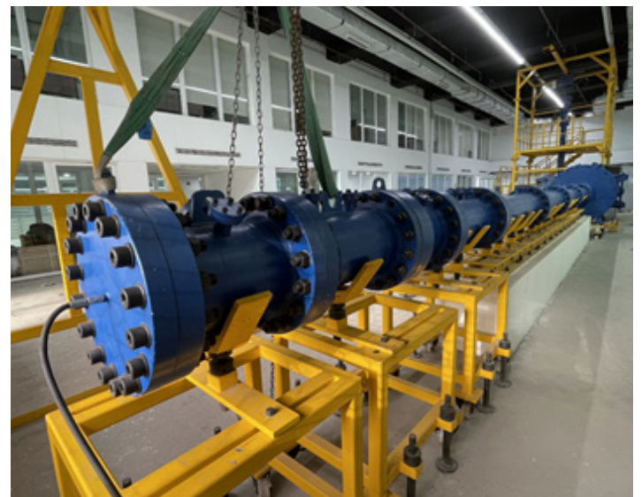
Fig 2: Horizontal shock tube test facility.
